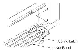
Figure 40 - Removing Louver Panel
